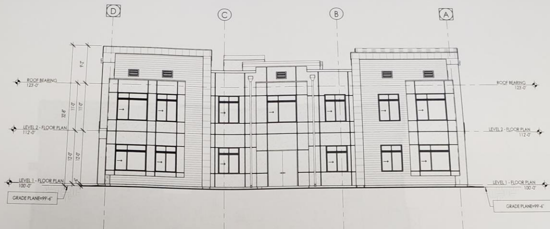
RIGHT (SOUTH) ELEVATION CODE REVIEW 1/8" = 1'-0"
