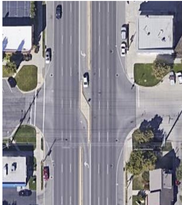
An example of the “super street “ concept that restricts left and though movements from cross streets onto a major street.
