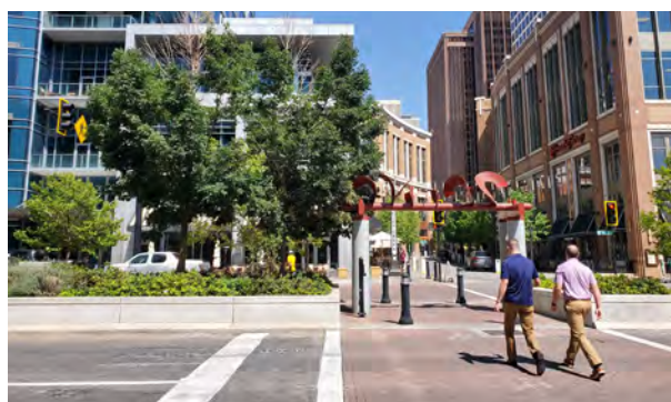
A center median in a downtown area can provide multiple functions - establishing a pedestrian refuge for pedestrian crossings while calming traffic, managing access, and greening the street, such as in this example from downtown Salt Lake City.
