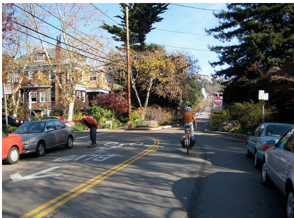
Bicycle boulevard treatments include traffic diversion, calming and speed reduction, and wayfinding signage, among others
