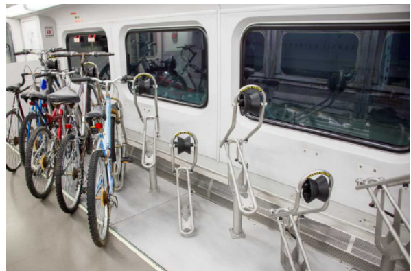
UTA's new 15-bike racks on FrontRunner will improve bike stability, avoid damage, and aid in easy removal. They will be tested and implemented in 2016 (Photo: Utah Transit Authority)
